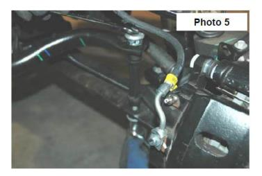
7. Using a 15mm wrench remove the bolts from the bottom strut mount.
