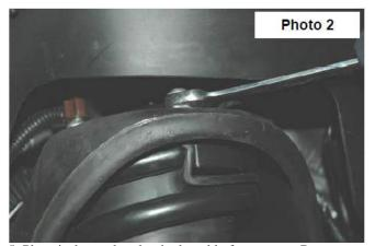
5. Place jack stand under the knuckle for support. Remove upper ball joint nut, using a 18mm wrench. Using a hammer hit the knuckle as shown to allow the ball joint to separate from the knuckle. See Photo 3.
