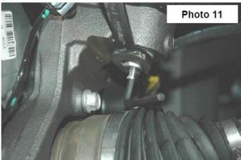
14. Reinstall the steering linkage nut using a 21mm wrench. If ball joint turns while tightening, use a 10mm wrench to hold the bottom of the tie rod.
