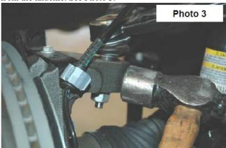
Do not allow the knuckle to pull out far enough that it pulls the shaft out of the differential.
