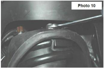
13. Raise the lower control arm and connect the upper ball joint on the upper control arm to the spindle. Using a 18mm wrench, torque to manufacturer specs.
